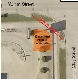
the city has determined the need to retain a 10-foot wide easement over this storm sewer, as shown in the illustration to the right. This easement is essentially 5 feet on both sides of the storm sewer pipe. The remaining portion of the existing easement may be vacated for the new bank facility.
